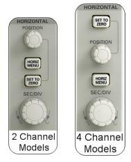
Figure 4.1: The HORIZONTAL control sections
