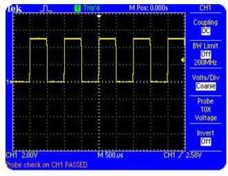
Figure 2.5: CH1 probe compensation signal
