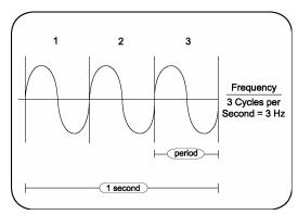
Figure 1.12: Frequency and period of a sine wave
