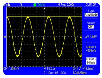
Figure 6.9: Volts/amplitude measurement for a 5 kHz sine wave
