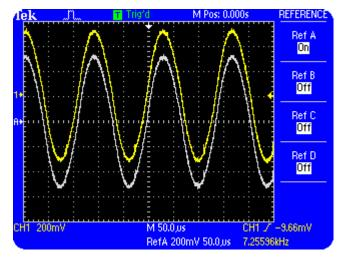
Figure 6.17: Reference waveform and updating waveform displayed
