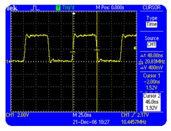
Figure 6.11: Pulse width measurements of a 10 MHz data signal using cursors
