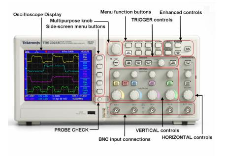
Figure 2.2: The TDS2024B digital storage oscilloscope
