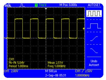
Figure 4.2: TDS2000B horizontal setup
