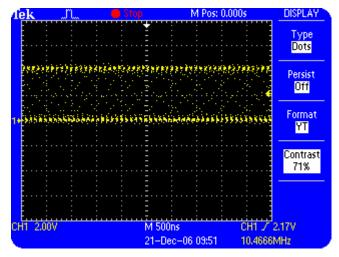
Figure 6.5: Waveform displayed in dots
