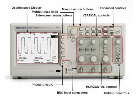
Figure 2.1 shows a TDS1001B digital storage oscilloscope.
