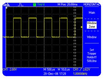
Figure 4.4: Position delayed and Window Zone
