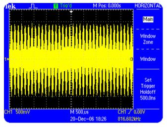
Figure 5.11 shows the updating overlay of the amplitude modulation region of an amplitude modulated (AM) signal.
