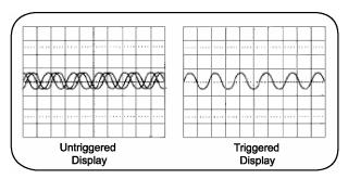
Figure 1.4 shows untriggered and triggered waveforms.
