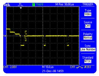
Figure 2.14c: Triggering on video lines
