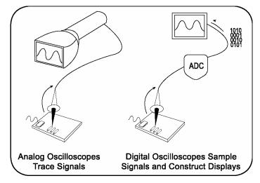
Figure 1.2: Analog and digital oscilloscopes
