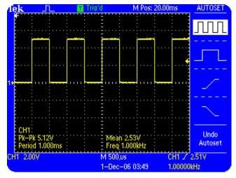
Figure 4.3: Delayed trigger position for a waveform
