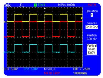
Figure 3.4:Display of CH1+CH2
