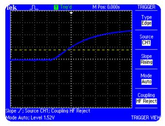
Figure 5.3: Triggering waveform with HF Reject coupling
