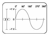
Figure 1.13: Phase in a sine wave
