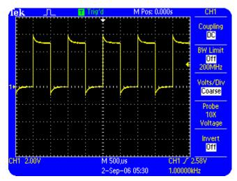
Figure 2.7: Probe overcompensated
