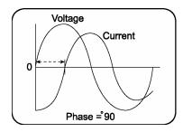
Figure 1.14: Phase shift between two sine waves
